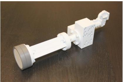
This is a Ka Satcom Transmit/Receive scalar feed providing high isolation and very low return loss. Both ports cover the whole range from 17.2 GHz to 31 GHz. This delivers a huge amount of flexibility allowing Elite to offer a variety of configurations including a 4-port feed from the same design. Both ports can be set as Receive ports or both as Transmit ports.
