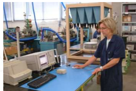
Final test with network analyzer
