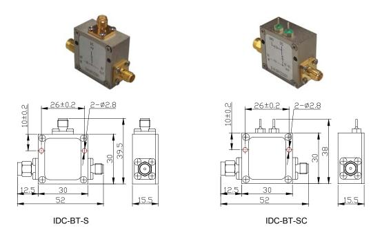
IDC-BT-X-S Bias Tee provides both DC bias current and RF signal via bias network. The features include small size, light and flat frequency response, it is used in microwave measurement area such as amplifier, programmable attenuation and switch circuit etc.
