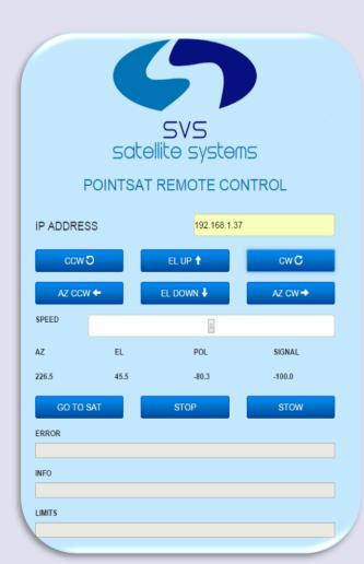
The latest antenna controller version of SVS, Pointsat allows you to control antenna via Android based devices or PC through ethernet cable.
